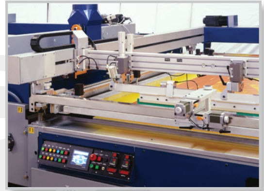
Servo-driven carriage ensures accurate, smooth travel
