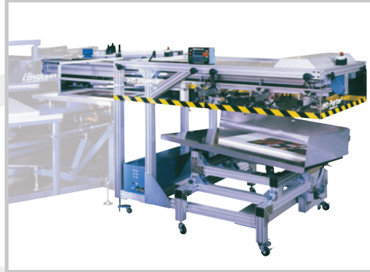
M&R's Porter™ is a fully adjustable suction-style takeoff that adapts to virtually any substrate (sold separately)
