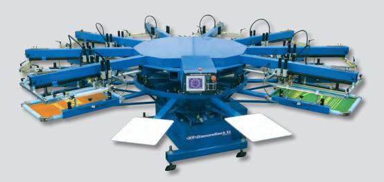
Diamondback XL automatic screen printing press combines servo drive, large image area, and affordability. Diamondback XL is available in 8 and 9 colors. It has a maximum image area of  $51 \times 53$  cm ( $20" \times 21"$ ), and can accept screen frames up to  $66 \times 91 \times 4.5$  cm ( $26" \times 36" \times 1.75"$ ). It's the ideal press for large images at a low cost.
