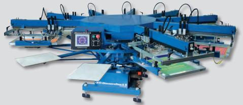
Diamondback S automatic screen printing press was the first press to bring servo drive to the entry-level user. It's available in 6, 7, 8 or 9 colors. It has a maximum image area of 41 x 46 cm (16" x 18"), and can accept screen frames up to 58 x 84 x 4.5 cm (23" x 33" x 1.75"). For those waiting for the right price on an entry-level automatic, the wait is over.
