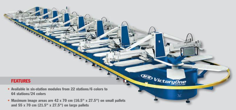
Servo-driven indexer and electric printheads provide exceptional smoothness, consistency, and longevity
